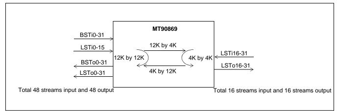
Figure 5 - 12K by 4K Blocking Configuration
