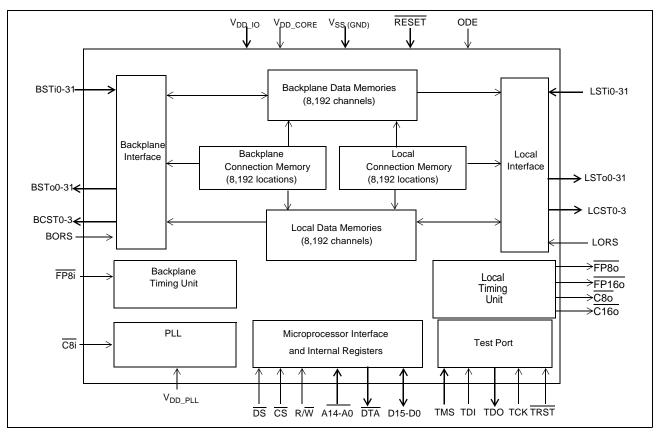
Figure 1 - MT90869 Functional Block Diagram
