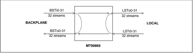
Figure 3 - 8,192 x 8,192 Channels (16Mb/s), Bidirectional Switching
