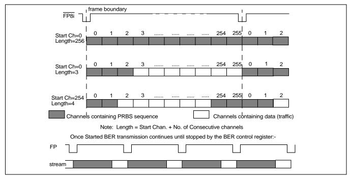
Figure 17 - Examples of BER transmission channels
