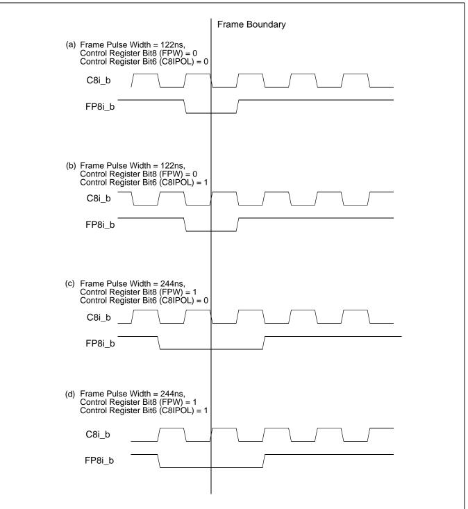
Figure 18 - Frame Boundary Conditions, ST- BUS Operation
