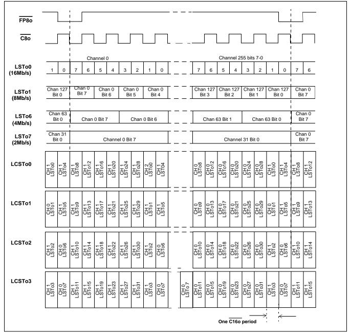
Figure 13 - Local Port External High Impedance Control Bit Timing (ST-Bus mode)
