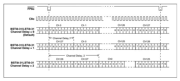
Figure 9 - Backplane and Local Input Channel Delay Timing Diagram
