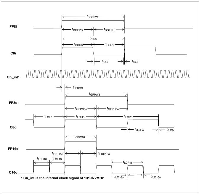
Figure 21 - Backplane and Local Clock Timing for GCI-BUS
