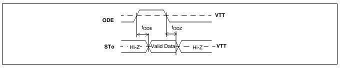
Figure 29 - Output Driver Enable (ODE)
