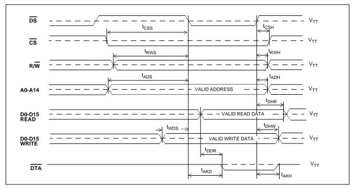
Figure 30 - Motorola Non-Multiplexed Bus Timing
